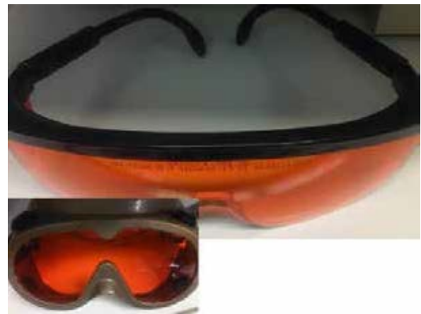
Figure 4. The goggles have a label on its lens or frame indicating the optical density for each wavelength range. Each person is responsible for confirming that the goggles are appropriated for the laser wavelength in use and has correct optical density that allows adequate ocular protection. The colors of the glasses do not confer any secure indication, only the label on the goggles can do it.
