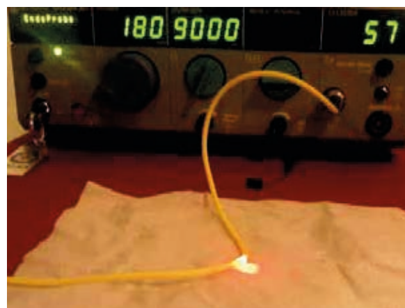
Figure 2. A broken optic-fiber. Note the output of the laser beam from the broken point of the optic-fiber.
