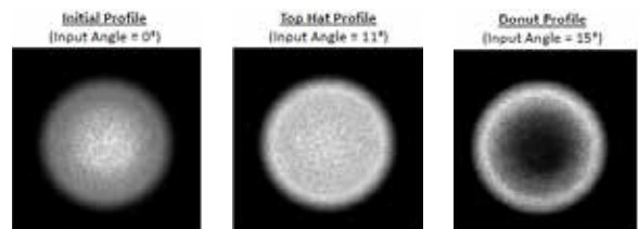
Figure 6. Modifying Beam Profiles with Multimode Fibers 13 . By increasing the launch angle of a Gaussian beam into a multimode fiber, the output beam profile can be modified. As the input angle was increased, the proportion of meridional rays to skew rays increased, firstly, forming a top hat and then a donut beam profile 14 . The top hat profile has a squarer wave appearance and allows for a more continuous and homogenous distribution of the photothermal energy throughout the entire spot area. This avoids Bruch's membrane rupture with short pulses.
